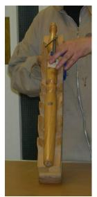
The drilling is done on a pillar drill, using a series of Vee blocks, with the workpiece clamped securely in place. Before doing the drilling, check and re-check that you are drilling the holes in the right place, as you've invested a lot of time and effort in getting the wood into shape and you wouldn't want to get it wrong, especially with ladies and small children present.
