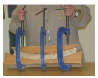
When removing the wood, your glasses will steam up instantly allowing people to sneak into the workshop and steal your biscuits, so remove your glasses. Clamp the wood into the jig as quickly as possible.
