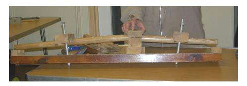
If you are forming the spindle set for the back of the chair, make sure that you glue them into position as soon as you remove them from the former, so that they restrain each other from bending back out of shape. Anne recommends Cascamite Resin Wood Glue, which I found on Amazon in various sized tubs.
